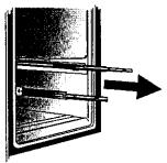
While supporting door, hook door supports into tabs located on inside of rail.
